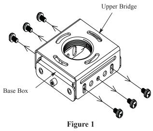
1. Separate the Upper Bridge from the Base Box by removing the six (6) M6 x 12mm Phillips Head screws three on each side (Figure 1).
